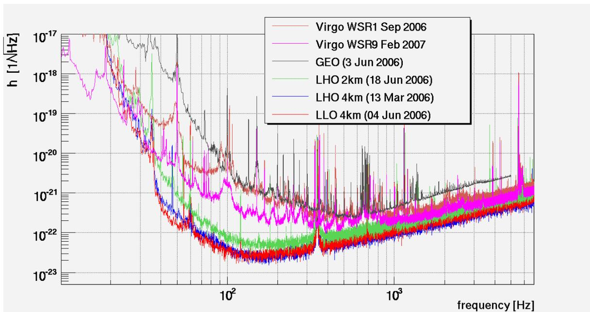
*Figure 1: Virgo sensitivity during WSR1 and WSR9 compared to the LSC detector sensitivities running at the same time.*
