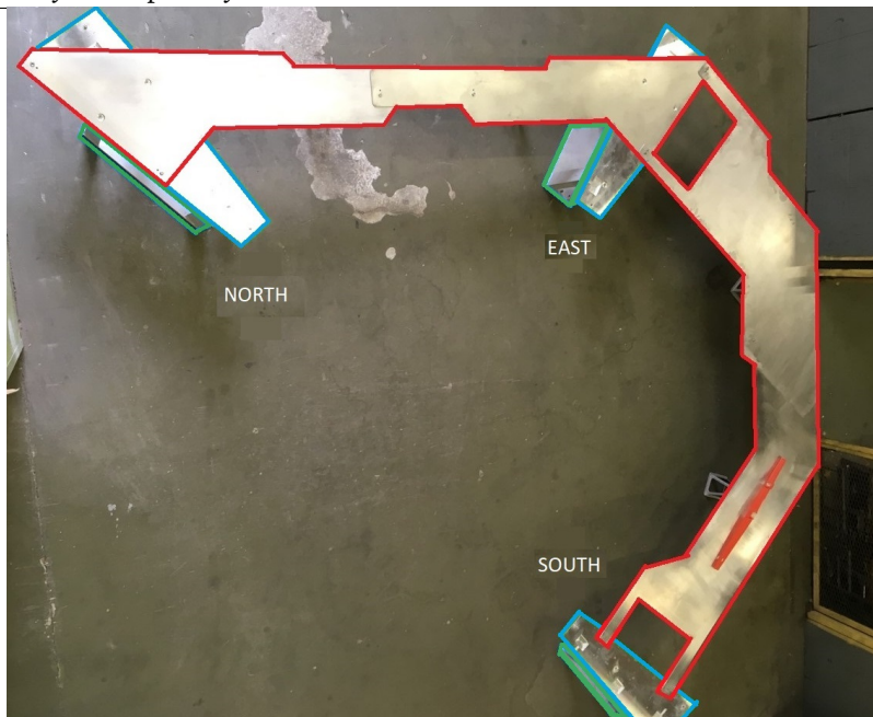
Figure 4: Top view of the complete assembly done at IPHC. In red is shown the aluminum template made of four plates used for the positioning, in blue are shown the aluminum reference plates and in green are the aluminum supports for the NCal.
