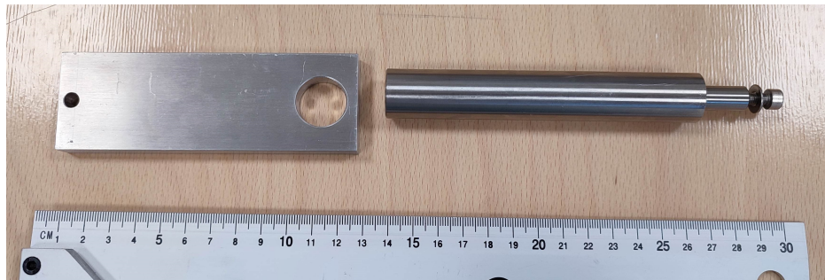
Figure 4: The two parts of a template used. On the left is a small aluminum plate on the right is a metal bar.
