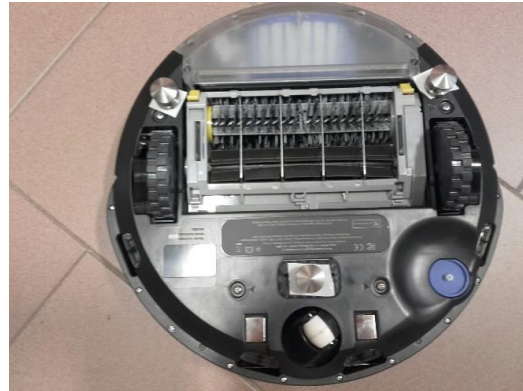
Right: Roomba bottom with 3 steel conical tips attached.
