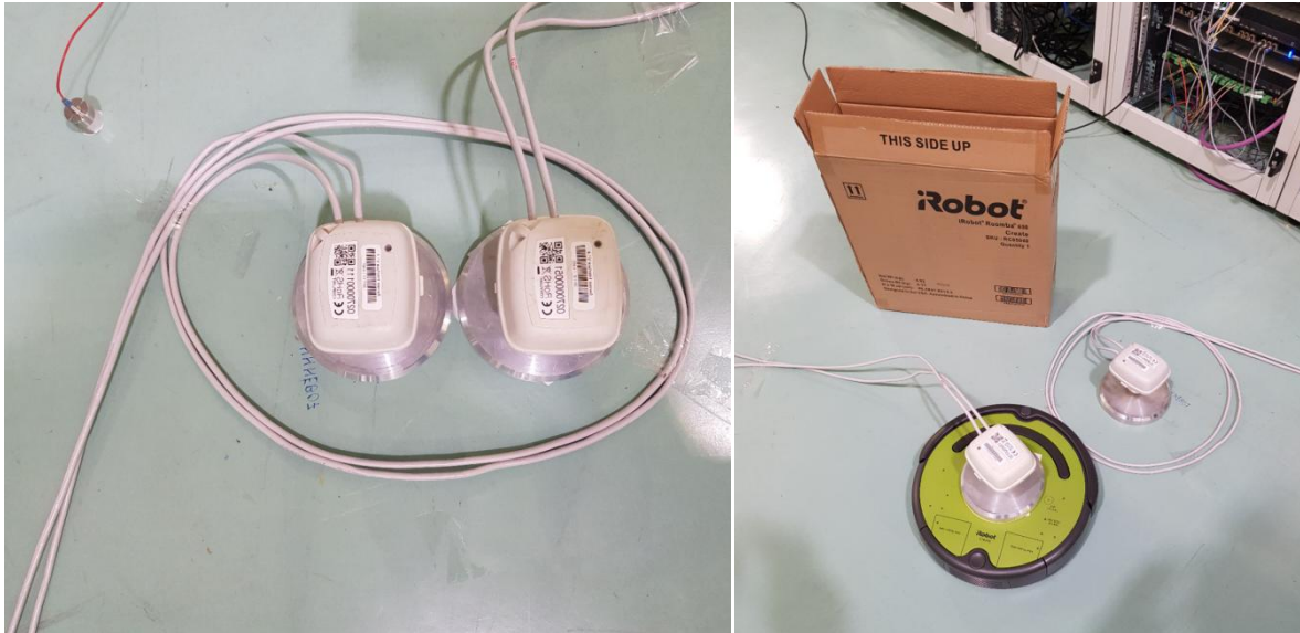
Figure 1. Pictures of the setup at Virgo North end experimental building (NEB). Left: Huddle test of two Innoseis geophones, both attached to the NEB concrete floor with double side tape. Right: one Innoseis sensor is attached on the Roomba platform using double side-tape.
