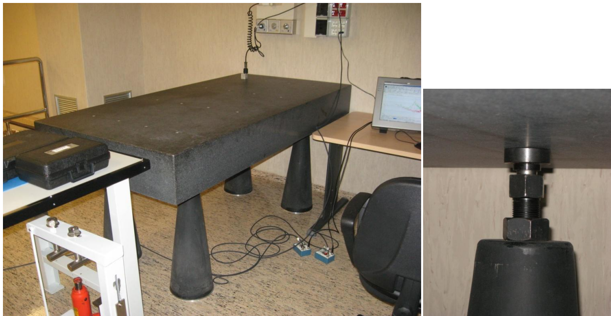
Figure 1. (left) picture of granite bench; (right) detail of support leg contact point.
