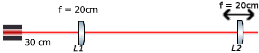
Figure 17: The setup of an optimization usage of theia , the position of L2 is varied in order for the waist of the final beam to be as large as possible.
