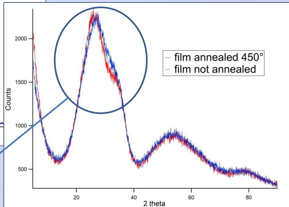
The diffraction pattern of the annealed sample is sharper than the not annealed one
