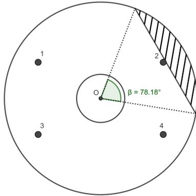
Figure 3: Outline of the counterweight for R4-03. The hatched area represents the material removed.
