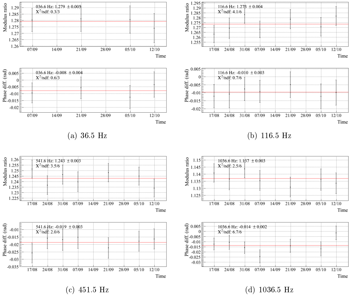
Figure 15: Evolution as function of time of the measured actuation TF ratio (LN1/HP) for the left coil of the WE mirror at four different frequencies.
