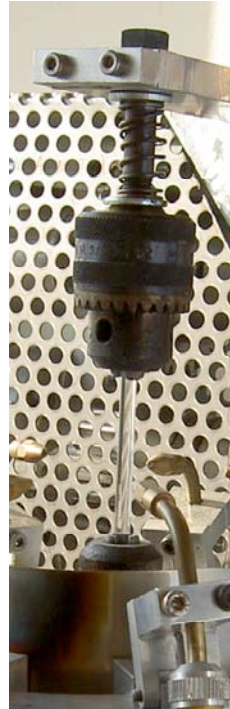
Fig.4-The two mandrels clamping the rod.
