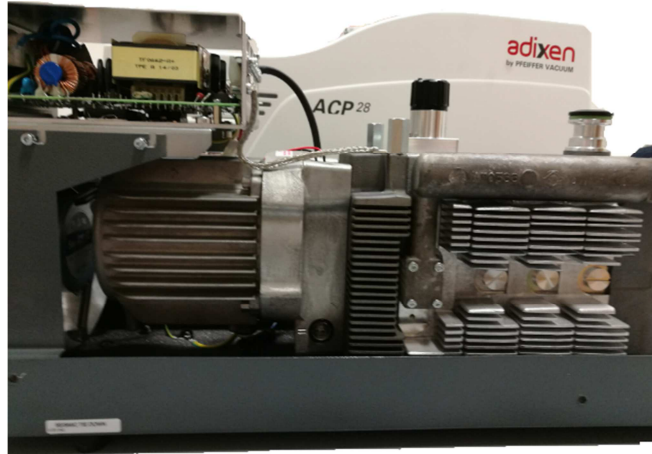
Figure 17: a multistage root pump being considered for the towers service
