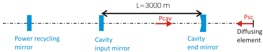
Figure 1: Double cavity configuration of the Virgo interferometer.
