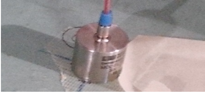
FIG. 9: Wilcoxon Meggit-731 accelerometer affixed to WEB floor
