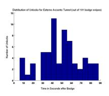
Figure 2: This plot shows the IMC power during the 60 seconds after each badge swipe at the "Eastern Accanto tunnel" door. The graphs for all badge swipes are overlaid. Note that the number of unlocks increases 30 seconds after the badge time.
