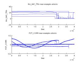
Figure 4: Plots of the Master Laser PZT Correction and the IMC Power in the 2 seconds surrounding an unlock, for five randomly selected example unlocks for which the PZT saturated. The five examples are overlaid. Note that the unlocks are fast, sharp drops.
