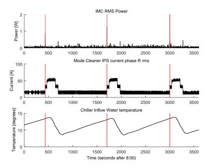
Figure 10: Correlation between chiller and IMC misalignments, shown for 8:00 - 9:00 UTC, 13 June 2015. Red lines mark the times of misalignment. top panel: Mode Cleaner power in trend data. middle panel: Mode cleaner building interruptible power supply current. lower panel: Mode cleaner building chiller water inflow temperature.
