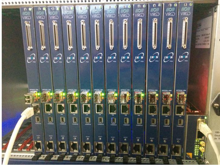
Figure 1: 12 Udspt boards in a uTCA chassis. On the right, the NAT-MCH switch. There are 800 GFLOPS available inside the chassis.
