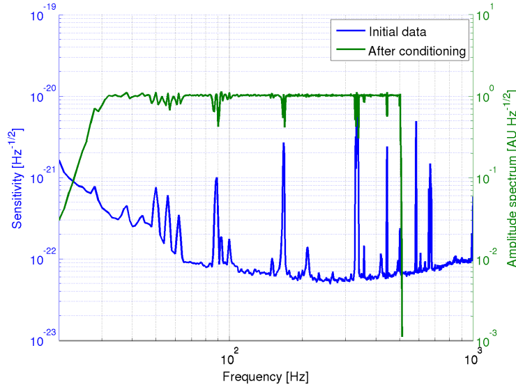
Figure 7.4: Shown is the amplitude spectral density of real Virgo data with a 1 Hz resolution before and after the data conditioning procedure described in the text. The blue line shows the amplitude spectral density of the data collected by the detector. The green line shows the conditioned data with an arbitrary overall rescaling. The high pass filter clearly removes the data fluctuation below 30 Hz and the anti-aliasing filter above 500 Hz. The lack of frequency content above 512 Hz is due to the data down-sampling. The amplitude spectral density in between is flat with the exception of frequency ranges that contained lines, these frequency ranges see their contribution downgraded which is not detrimental to the analysis as the detector does not have a good sensitivity at these frequencies.
