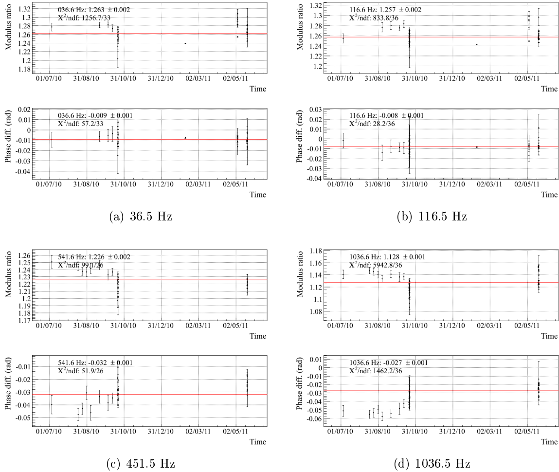
Figure 1: Evolution as function of time (June 2010 to May 2011) of the measured actuation TF ratio (LN1/HP) for the up coil of the WE mirror at four different frequencies.
