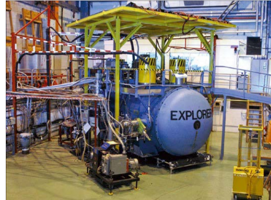
EXPLORER resonant bar operated @ CERN 1991-2012
