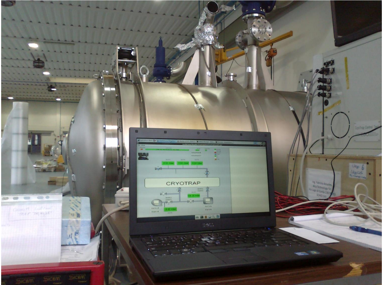
Figure 2: Synoptic used to Control the cryotrap
