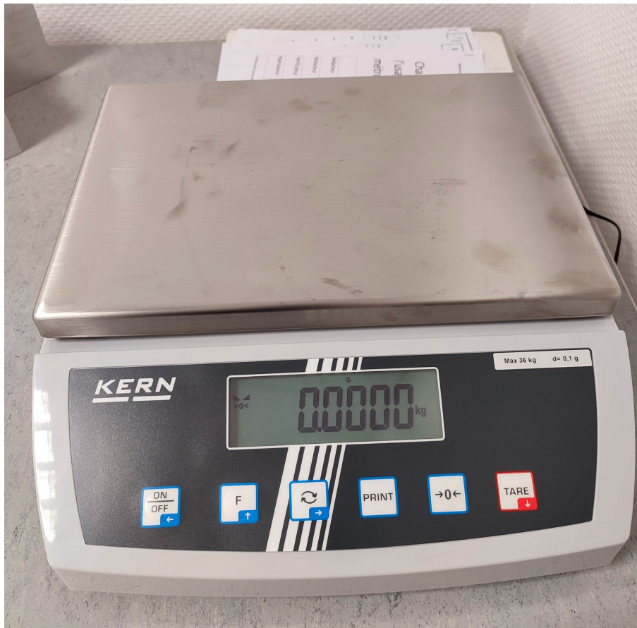
Figure 15: Scale used to measure the mass of the cylinder. The model is a KFB 36K0.1.
