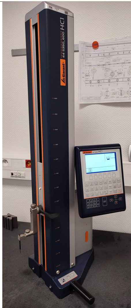
Figure 17: Measuring column used to measure the diameter and height of the cylinders. The model is a Garant 44 5350_600 HC1.
