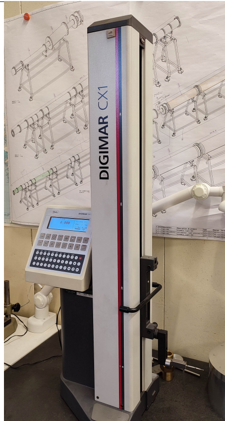
Figure 18: Measuring column used to measure the diameter and height of the cylinders. The model is a Mahr CX1.
