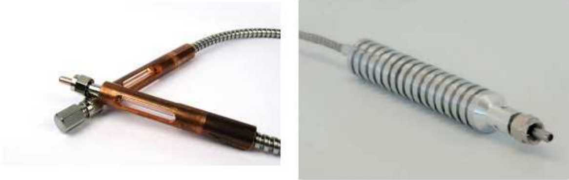
Figure 3.1: The two high power connectors that were used in our experiments. The high power SMA-905 connector on the left furnished with the fibers from NKT photonics and the SMA-6 connector developed by Alphanov.
