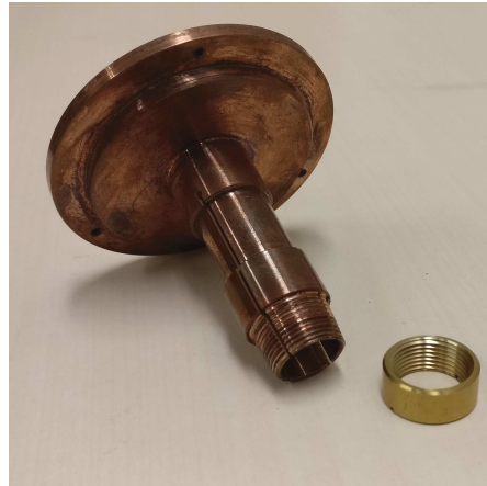
Figure 5.18: New holder for the magneto-optical crystal. Its conic outer diameter allows to control the stress applied on the crystal while screwing the ring
