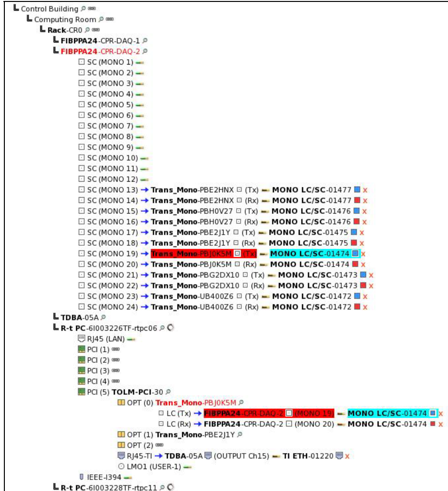
Fig.1: Logical tree representation of part localization using the self container-contained relational concept. In addition, an optical fiber connection logical representation is shown between a patch-panel and a TOLM-PCI. The TOLM_PCI part occupies a PCI slot of the R-t PC, the Trans-Mono part occupies an OPT slot of the TOLM-PCI, and the cable MONO LC/LS occupies an LC connector of the transceiver Trans-Mono.
