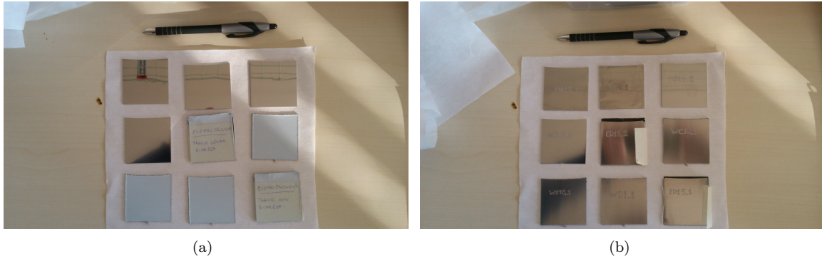
Figure 10: Stainless steel substrates before sending them to Entegris for coating. (a): Front, some of the samples underwent cleaning at EGO, some others were sent with the original protective film. (b): An identity code was etched on the back of the samples.
