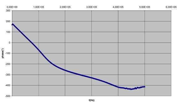
As the phase decreases linearly with the frequency, the delay of the filter is constant and is about *6,8µs* before the cut-off frequency. Of course this delay does not include the compression inversion (-180°).
