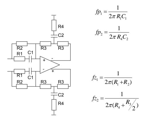
Following, the transfer function of the compression filter for 2Hz-12Hz filtering. Gain unit is normalized to 1 in the low frequencies domain. To fit to the ADC input dynamic range, the gains are  $\frac{1}{4}$  to 9 before and after the cut-off frequencies.
