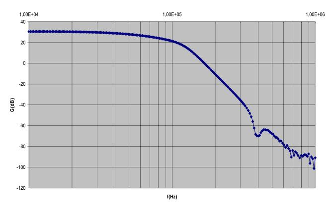
The low frequency gain is 30dB because we used the compression input stage with a 30dB gain in order to cover the analyzer dynamic range. The cut-off frequency is 100kHz (g=-3dB). At the Shannon frequency the gain is -70dB which represents a -100dB rejection with the use of notches. With not, the rejection is about -90dB.
