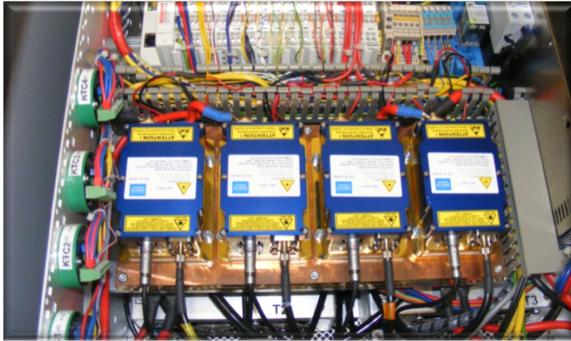
4 pumping fibered 10-12m laser diodes
