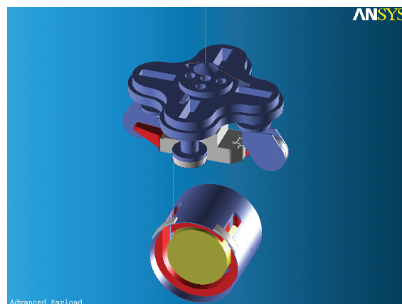
Figure 35: Schematic picture of the new payload in the configuration with the marionette reaction mass is adopted.
