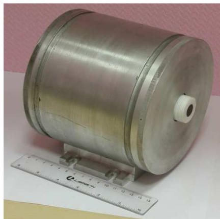
Figure 40: Photo of the FI magnetic system in s case
