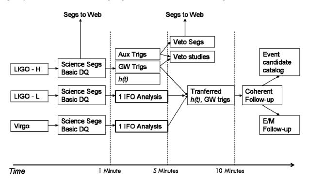
Fig. 1: Diagram of the burst online analysis proposal [1].
