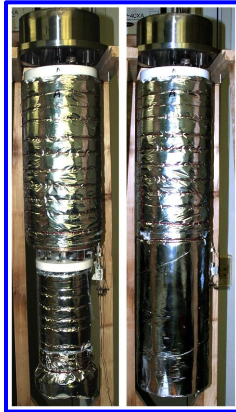
LN2 (top) and Lhe (bottom) chambers
