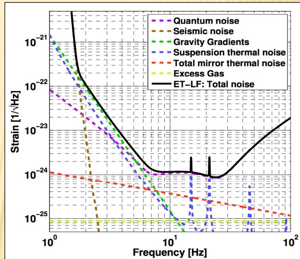
As mirror TN is no longer limiting, one could relax the assumptions on the material parameters and the beam size...
