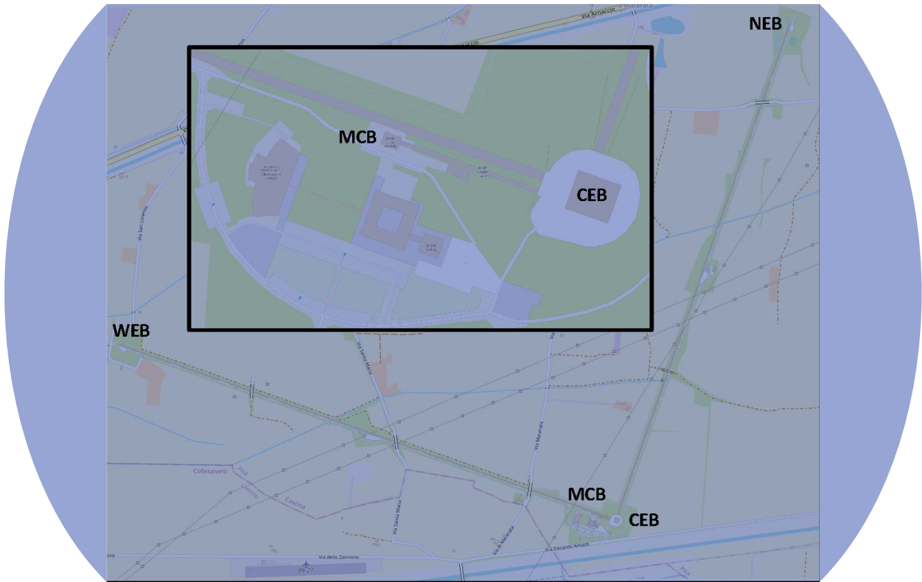
Figure 2: Map [21] of the EGO site showing the Virgo detector and in particular the location of the main buildings identified in the text. The central insert shows a zoom around the interferometer vertex, with the CEB and the MCB highlighted. The Mode-Cleaner cavity is 144 m-long while the Virgo arms are 3-km long.
