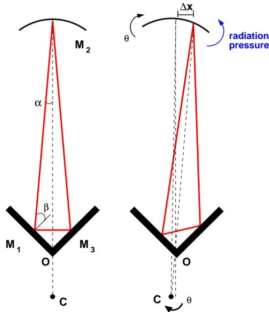
Figure 1: Effect on the translation of the beam in a triangular cavity due to the misalignment of the terminal mirror. The beam will meet the terminal mirror following the straight line which connects the center of the dihedron, O, and the center of curvature, C.
