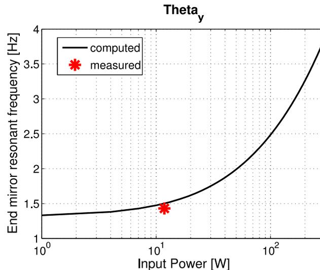
Figure 2: Resonant frequency of the IMC terminal mirror as a function of the input power. The behaviour obtained with the analytic computation result to be quite in agreement with the measured resonant frequency, red star.
