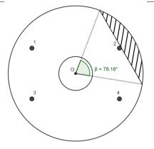
Figure 3: Outline of the counterweight for R4-03. The hatched area represents the material removed.
