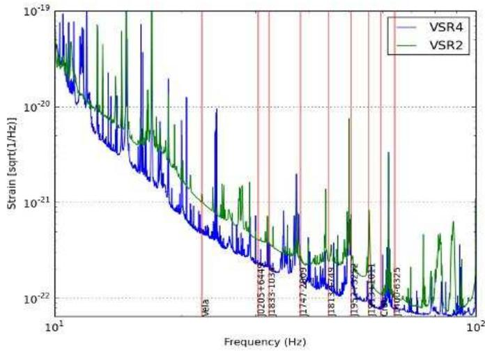
Figure 2 : VSR2 (green) and VSR4 (blue) sensitivity curves at low frequency.
