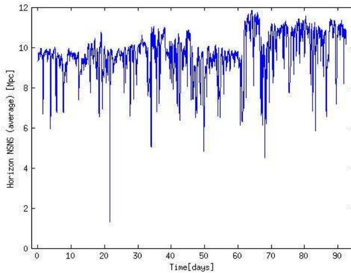
Figure 1: Horizon (distance at which a neutron star binary coalescence is observed with a SNR of 8 in the Virgo detector) as function of time during VSR4.
