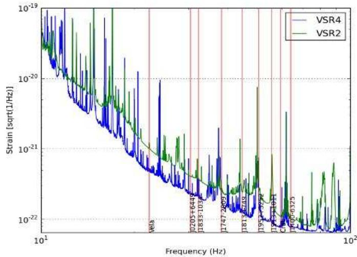
Figure 2 : VSR2 (green) and VSR4 (blue) sensitivity curves at low frequency.
