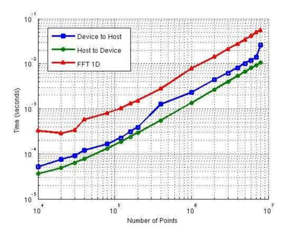
Fig. 5: PCIe bus data transfer latencies contribution to the FFT 1D calculation using CUFFT single-precision from CUDA.
