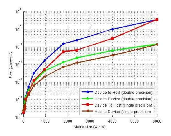
Fig. 2: PCIe bus data transfer latencies in both directions using CUBLAS on GPU using single and double precision.
