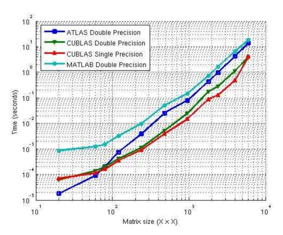
Fig. 1: Matrix multiplication parallel computation performances from Matlab (2009A) and ATLAS on CPU multi-core, compared to CUBLAS single and double precision on GPU.
