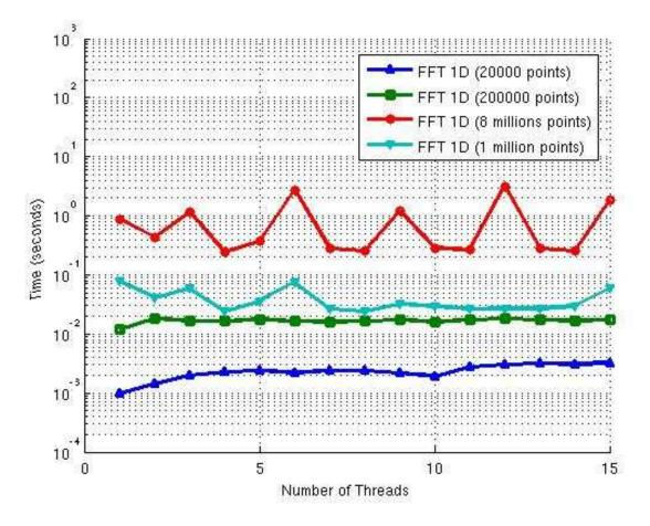
Fig. 3: FFT 1D computation performances of multi-threaded FFTW (on CPU) as a function of the number of threads used.
