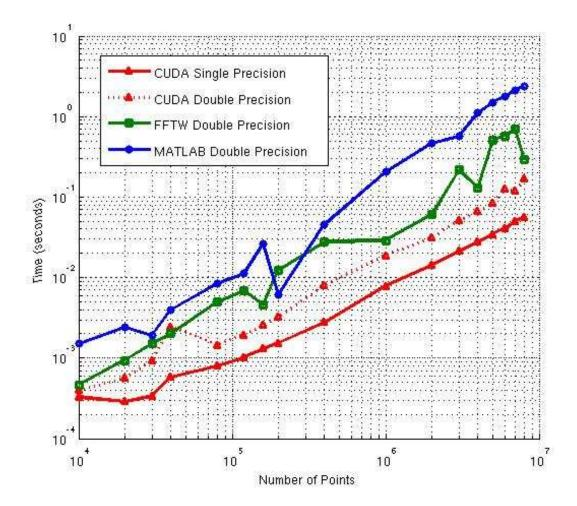
Fig. 4: FFT 1D performance comparison between CPU and GPU. For FFTW, the number of threads is adjusted manually to get the best result (between 1 and 10 threads). For GPU we use the CUFFT library from CUDA framework.
