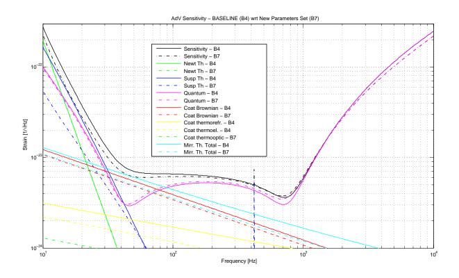
Figure 2: AdV baseline sensitivity from [1] (traces labeled B4, baseline scenario) and the new reference sensitivity, calculated with GWINC and using the parameter set described in Section 5 of this document (traces labeled B7, new reference scenario). The corresponding input files are IFOModel\_conceptual\_design.m for B4 and adv\_27062008.m for GWINC.
