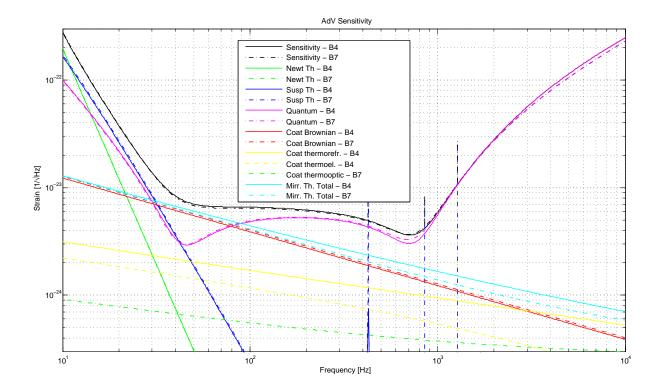
Figure 1: **Consistency scenario:** AdV design sensitivity calculated with BENCH version 4 (traces labeled B4, baseline scenario) and GWINC (v1) (traces labeled B7, consistency scenario). For both analyses the same set of input parameter (i.e. the set described in [1]) has been used.
