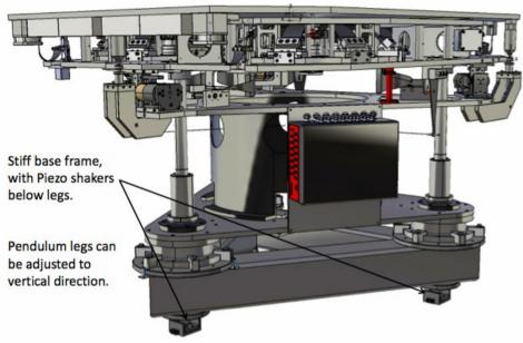
Install PZT based shaking system
