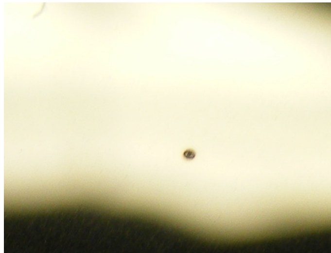
Figure 8: View of the damage created on SiC surface by Yag laser beam.
