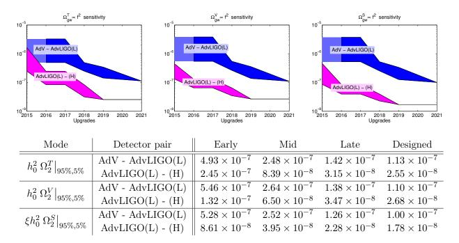
Figure 12: Upper limits for a stochastic background spectrum  $\Omega_{\text{gw}}(f) = \Omega_2 \left(\frac{f}{100 \text{ Hz}}\right)^2$ . The upper limit for the parameter  $\Omega_0$  is given as a function of the polarization, detector pair and epoch.
