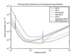
Figure 3: Data for the expected strain sensitivities at different stages of the upgrades are taken from [Aasi, 2013].
