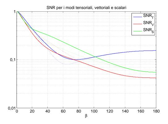
Figure 7: SNRs for different modes as a function of the separation angle  $\beta$  between the detectors. These functions are calculated for two different optimal configurations of the detectors' arms: solid lines are for Type I orientations and dashed lines are for Type II orientations (see Figure 5 for the definitions).
