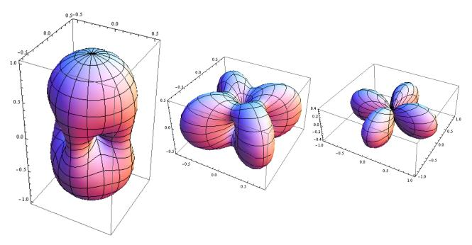
Figure 4: Angular pattern function for the tensor, vector and scalar modes, assuming no correlations between components. From left to right  $F^T = \sqrt{(F^+)^2 + (F^\times)^2}$ ,  $F^V = \sqrt{(F^x)^2 + (F^y)^2}$  and  $F^S = \sqrt{(F^b)^2 + (F^\ell)^2}$  are represented.
