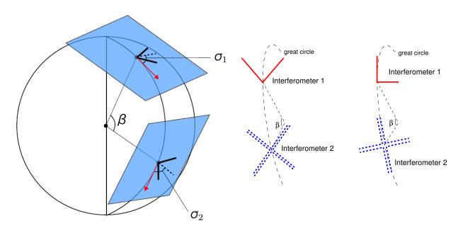
Figure 5: Coordinate system on the Earth for a detector pair. In the following we will distinguish between two particular orientations: the Type I (detectors' arms have the bisectors on the same plane, depicted in the middle) and the Type II (two arms of different detectors are on the same plane, depicted on the right).
