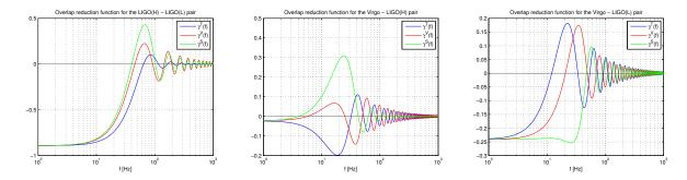
Figure 6: ORF for the different detector pairs Virgo - LIGO(L), Virgo - LIGO(H) and LIGO(H) - LIGO(L). Note how the difference of the behavior between the polarization modes appears at around the characteristic frequency  $f_c \equiv c/2|\Delta \mathbf{x}|$ , above of which the ORFs rapidly decrease to 0.
