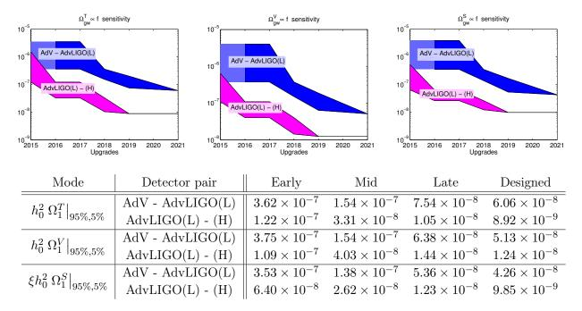
Figure 11: Upper limits for a stochastic background spectrum  $\Omega_{\rm gw}(f) = \Omega_1 \left(\frac{f}{100~{\rm Hz}}\right)$ . The upper limit for the parameter  $\Omega_2$  is given as a function of the polarization, detector pair and epoch.
