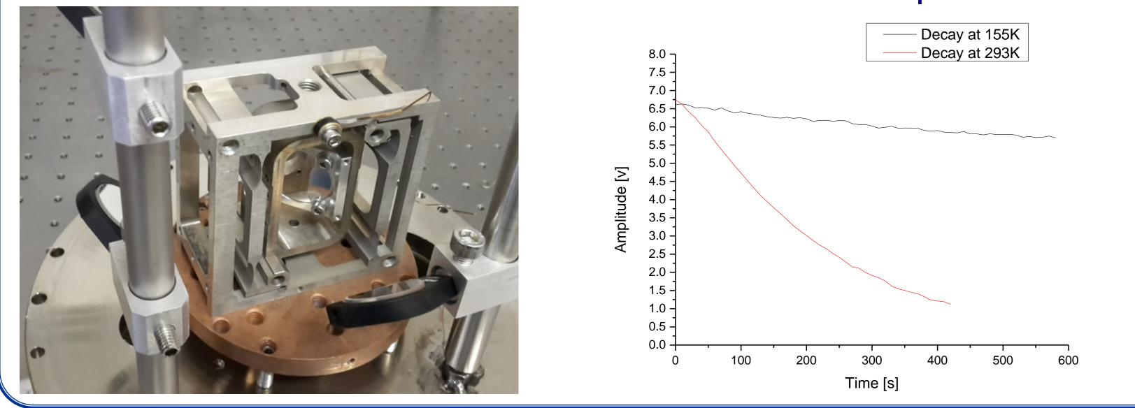
**Inertial mass oscillation amplitude decay** at different temperatures
