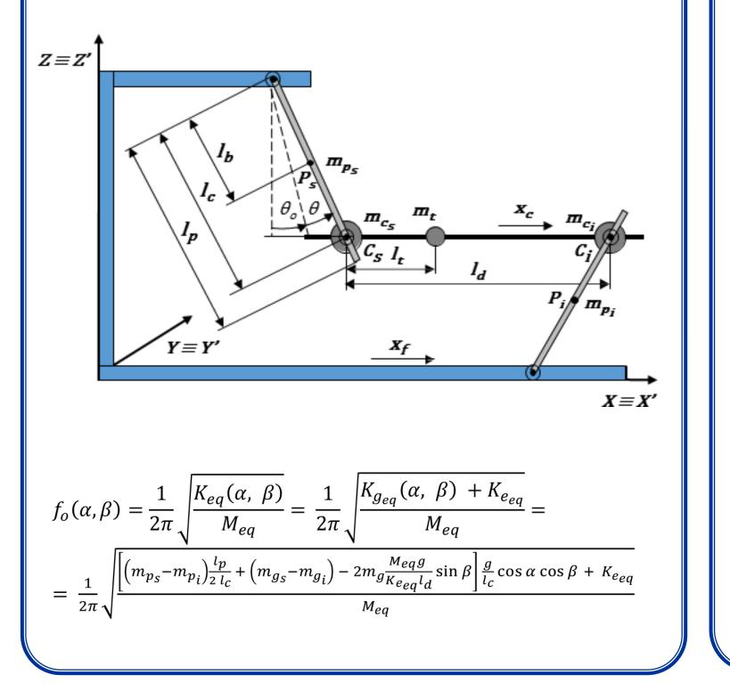
Scheme of the UNISA Folded Pendulum (Model GD14) with a shadow meter readout
