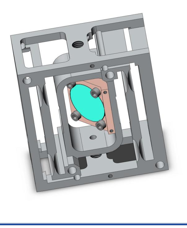
The folded pendulum mounted on the Perugia cryostat base, modified to reduce the recoil losses
