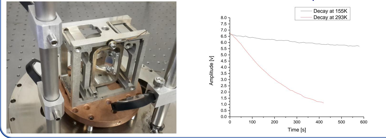
**Inertial mass oscillation amplitude decay** at different temperatures
