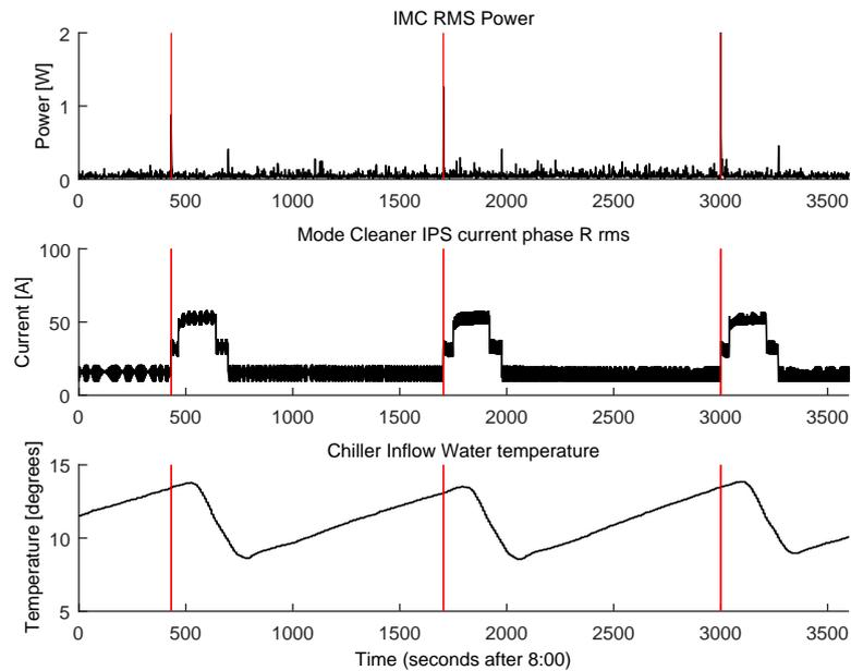
Figure 10: **Correlation between chiller and IMC misalignments, shown for 8:00 - 9:00 UTC, 13 June 2015.** Red lines mark the times of misalignment. *top panel:* Mode Cleaner power in trend data. *middle panel:* Mode cleaner building interruptible power supply current. *lower panel:* Mode cleaner building chiller water inflow temperature.
