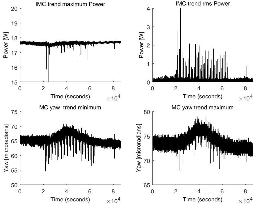
Figure 7: **MC mirror misalignments on 13 June.** Clockwise from upper left: Trend maximum power in the IMC. Trend rms power in the IMC. Trend maximum mirror yaw in the Mode Cleaner end mirror. Trend minimum mirror yaw in the mode cleaner end mirror. All plots are for the entire day of 13 June.
