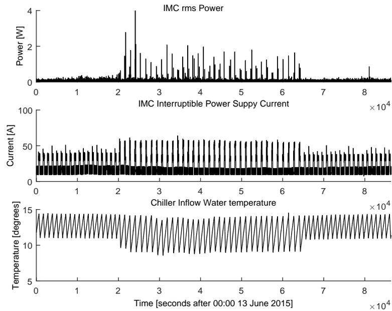
Figure 9: **Correlation between chiller and IMC misalignments, shown for 13 June 2015.** *top panel:* Mode Cleaner power in trend data. *middle panel:* mode cleaner building interruptible power supply current. *lower panel:* mode cleaner building chiller water inflow temperature.
