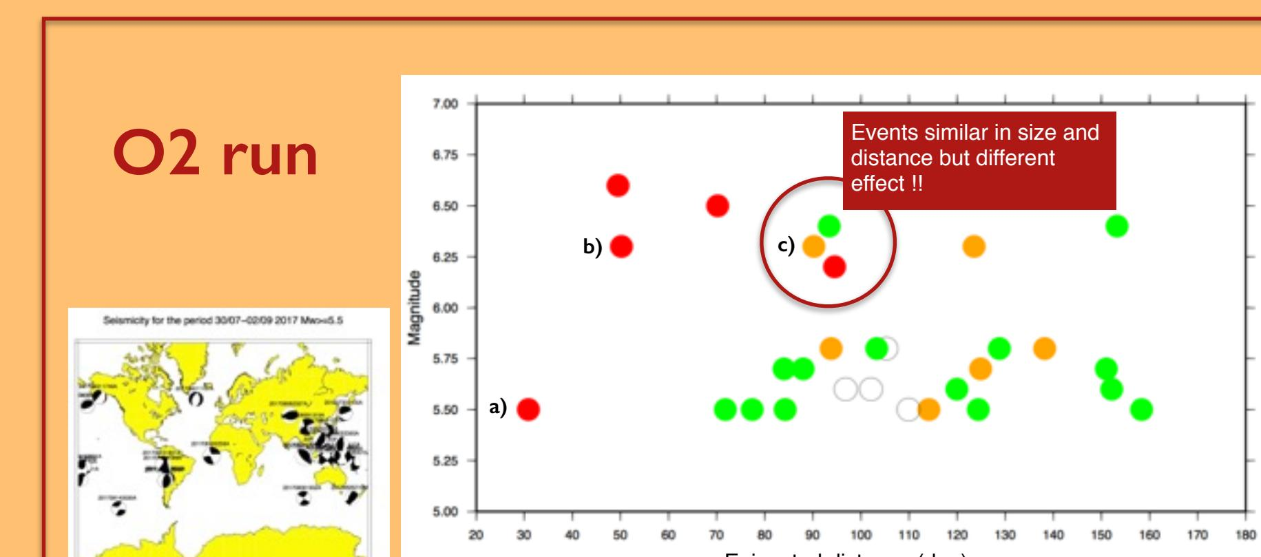
During the O2 run (30/07-02/09 2017) 30 earthquakes (Mw > 5.5) occurred (see above map with corresponding focal mechanisms). We evaluated their effects on the interferometer by means of the Hrec range that gives the instantaneous sensitivity of the interferometer in Mpc. Red dot = system out of lock, orange = sensitivity downgraded, green = no effects, open circle = no data. Examples are shown on the right column.
