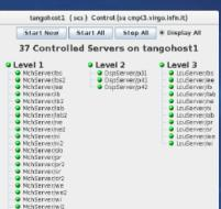
For initial AdV, software shall support about 150 boards. At system startup each board loads boot code via tfpt from a dedicated boot server. This code is actually a sort of basic OS. In a second phase software supervisor (based on software toolkit Tango Controls) downloads in each processor the hard real-time code.
