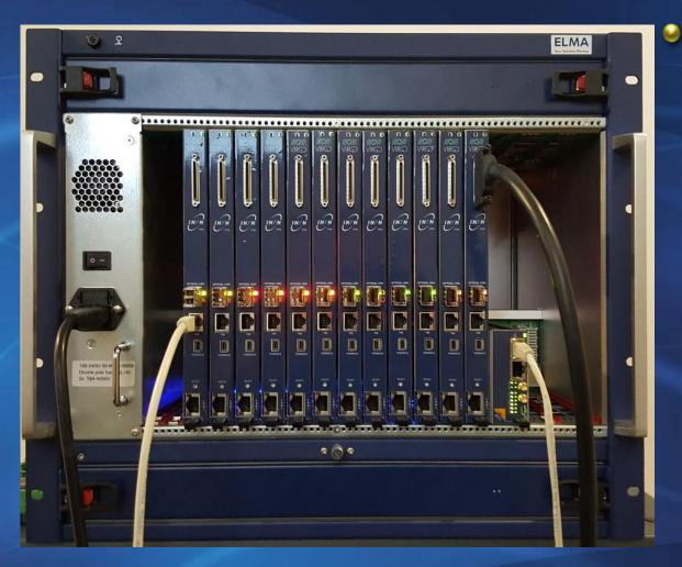
In a single 6U x 19" crate we can concentrate 72 ADC + 72 DAC channels supported by 720 GFLOPs, 12 x 1 Gb Ethernet ports + 12 x 1 Gb Optical Link for digital IO and a total power consumption less than 500 Watts
