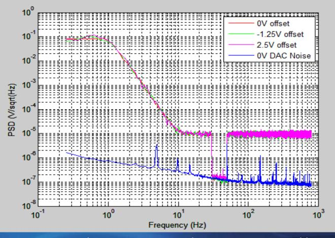
DAC output spectrum when converting a white spectrum signal low pass filtered (4 poles @ 1Hz + 4 zeroes @ 10 Hz) and stopband (30-50 Hz, Bessel 12th order,0.1dB ripple, -60 dB stopband). Signal amplitude was set to 0.6Vpp
