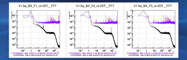
Performances tests on suspensions went beyond our expectation. Placing converters at front-end electronics level, together with introduction of digital demodulation, drastically improved noise immunity. Following picture shows improvement in vertical position sensors readout.
