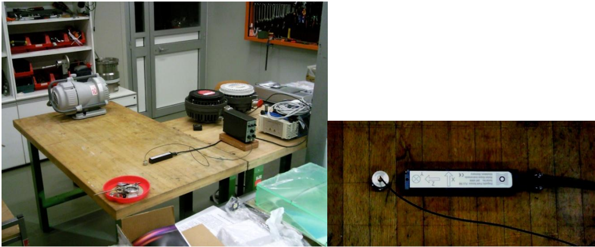
Figure 3. Setup 1500N. Magnetometer and seismometer lay on the wooden test bench, and are both feed on battery power. Signals are read and FFT computed with the onosokki spectrum analyzer. The measured source barycenter (scroll pump in this picture) is at about 1m distance from the probes. The source device is deployed on one custom seismic isolator made of three 1\text{cm}^3 pieces of sorbothane rubber ( http://sorbothane.com/ ) loaded with \approx 15\text{kg} weight. The measured resonance frequency of this isolator is around 7Hz.
