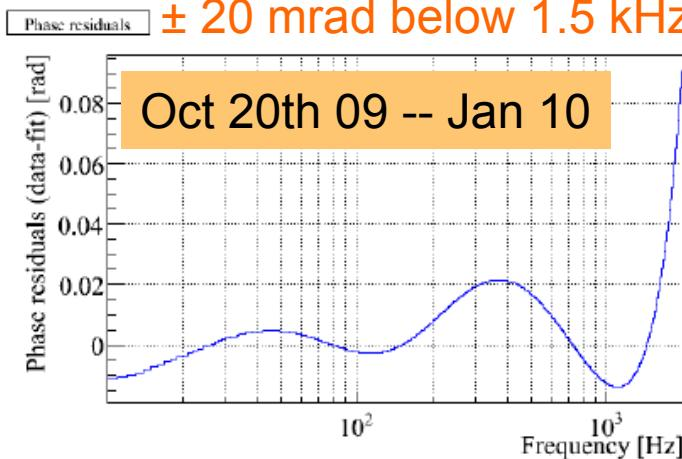
WE, L-R actuation uncertainties: 3% in amplitude, 20 mrad in phase and 10  $\mu\text{s}$  in timing
