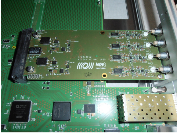
(a) DAC mezzanine prototype.
