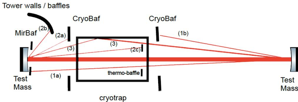
Figure 1: Re-coupling paths for scattered light (lengths not at scale). In this document we focus on path (1b).
