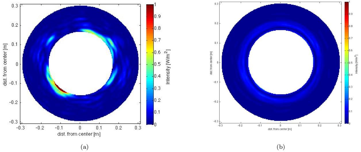
Figure 4: Distribution of power on mirror baffle for case1 (a) and case2 (b).
