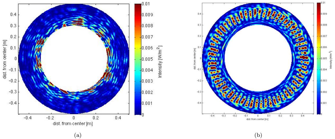
Figure 5: Distribution of power on CryoBaf for case1 (a) and case2 (b).
