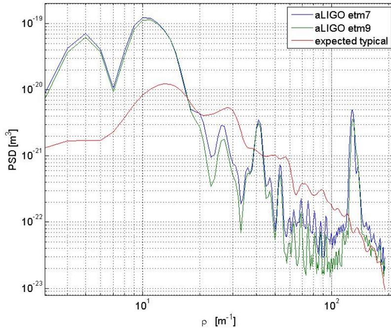
Figure 3: Measured PSD of 2 aLIGO ETM compared with a typical expected PSD in AdV that was used for calculating the requirements of SLC.
