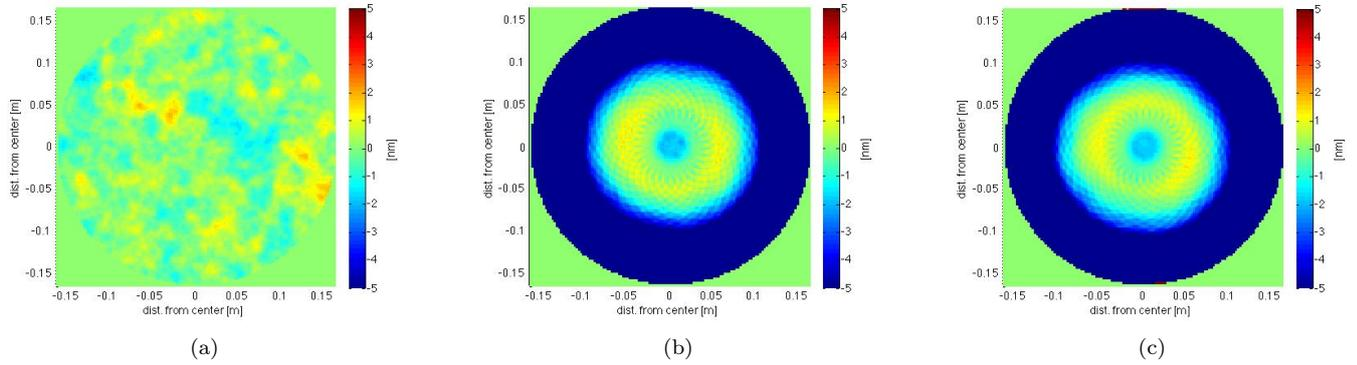
Figure 2: Typical expected mirror surface figure error with 0.5nm RMS (a), aLIGO measured mirror surface figure error of ETM7 (1nm RMS) (b) and ETM9 (0.9nm) (c).
