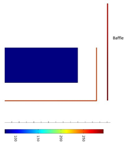
Fig.3 Case of Pyrex glass baffle (thickness 2mm). Temperature varies from -10°C at the exposed baffle edge to near room at the baffle outer boundary (respectively 263K to 290K in the sketch; the thermal shield temperature is about 245K)
