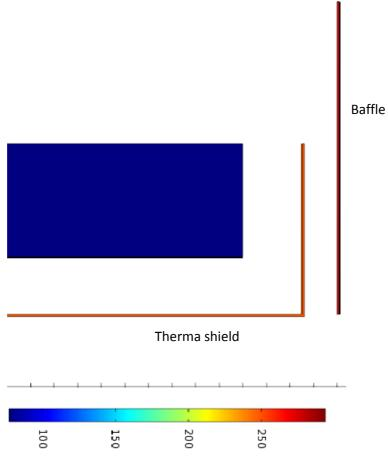
Fig.2 calculated temperatures, detail of the baffle (lower right corner of fig 1). Case of baffle realized in polished Stainless Steel (emissivity=0.1, thickness=2mm). The temperature of the baffle is around 272K, rather uniform.
