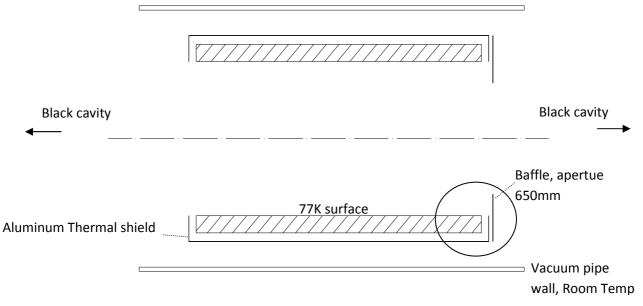
Fig.1 2D axial-symmetric sketch of tube cryotraps (2m long x 0.9m aperture) with one optical baffle at one extremity. The circled detail is the one reported in the next figures.
