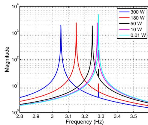
Figure 8: Mechanical Transfer function of the higher resonant mode  $\theta_x$  mode.
