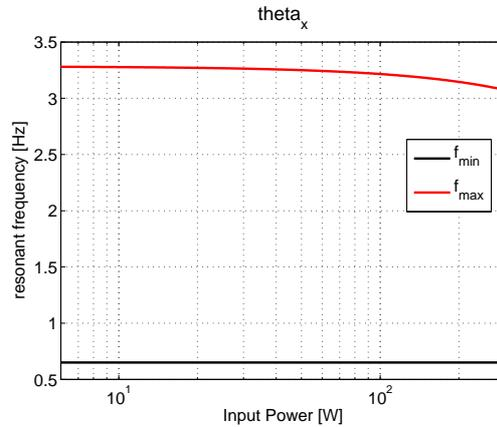
Figure 4: Effect of the radiation pressure on the system resonant frequencies, the 0.65 Hz frequency does not change due to the strong massivity of the injection bench.
