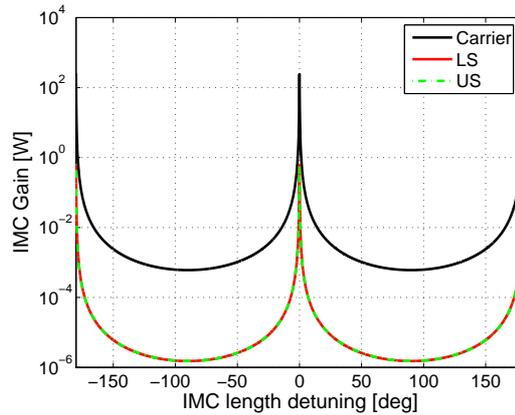
Figure 6: Sweep of the IMC terminal mirror along the  $z$ -direction in order to evaluate the resonant condition. The longitudinal position of the mirror has put on resonance and the cavity has a Finesse of about 1100.
