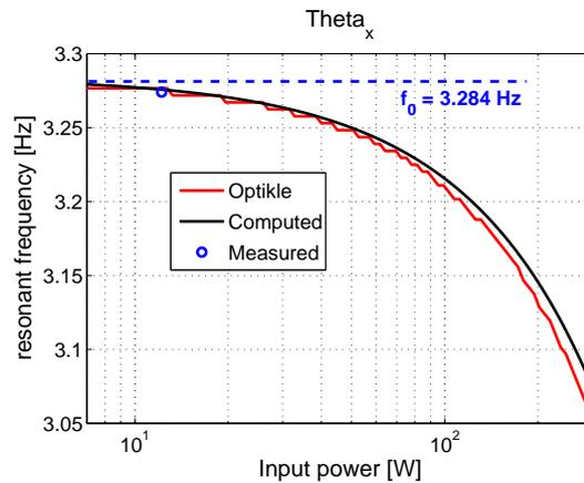
Figure 9: Higher resonant frequency behavior comparison between the result of the analytical computation and the simulation done with Optikle. It shows a very good agreement.
