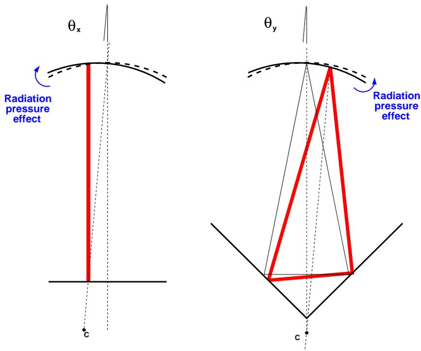
Figure 10: Effect of the radiation pressure in a triangular cavity on the  $\theta_x$  and  $\theta_y$  directions. The effect of the radiation pressure on the two directions is completely different: on the  $\theta_x$  the radiation pressure acts on the system lowering the stiffness, while on  $\theta_y$  the radiation pressure increase the stiffness.
