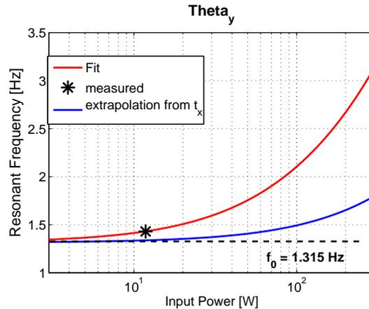
Figure 11: Radiation pressure effect on the IMC terminal mirror yaw direction.
